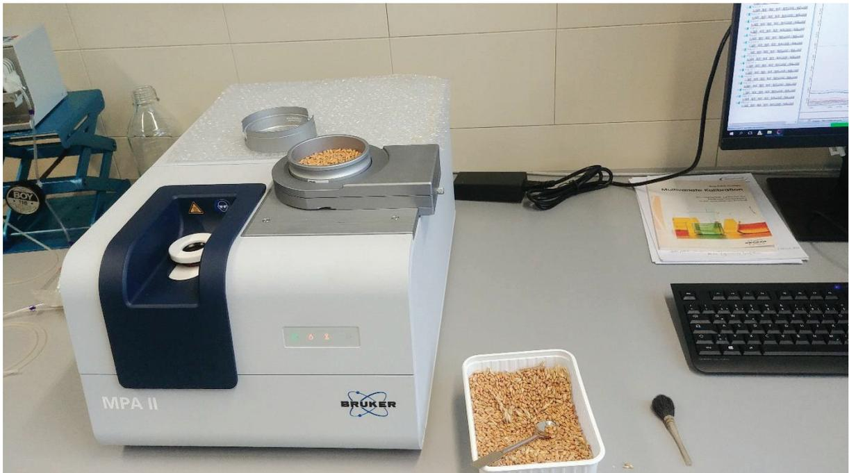
Abbildung A 5: Bruker MPA II NIR-Sensor
