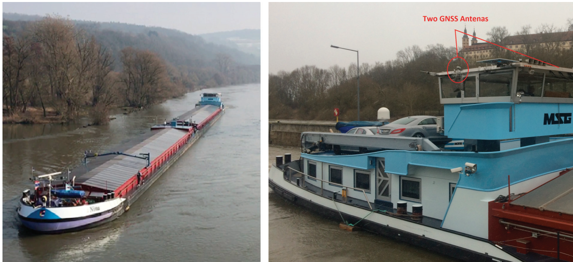
FIGURE 4.3: Vessel EL-NINO and the two established on-board GNSS antennas
