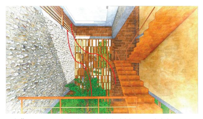
Stack effect is necessary to keep indoor ventilated. The skylight court inside the house is enhanced with an indoor tree and vents on the side allow the warm air to rise up and keep the interiors cool.
