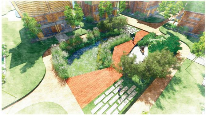
The eco courtyard acts like the space for stack effect and as a sponge for the rainwater to seep into. Excess rain can be stored in the mound temporarily and on most occasions, it acts as an open landscaped garden space. Each eco courtyard has no more than 8 units around it to keep the scale compact and promote social interaction amongst the house units.
