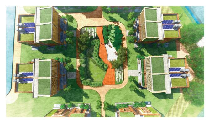
Individual cluster 3d view. Each house covered in green roofs. Solar panels facing the western side to absorb maximum sunlight. Two water tanks for grey water and drinking water.
