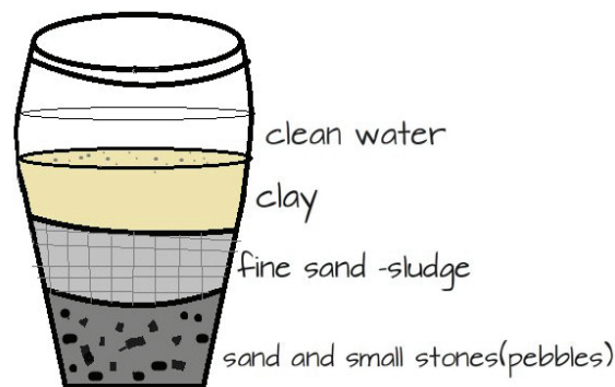
Figure 2.16: Cob Shake test ( http://www.buildNaturally.com/EDucate/Articles/Cob.htm )
