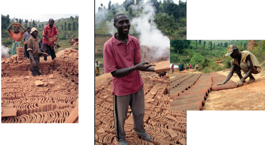
Figure 2.20: Mud bricks (Adobe), in different shapes for walling and roofing, let to dry in the sun. Rwanda-ActionAid school Project 2012 (Source: Personal archive of Thanos Bouziotopoulos)
