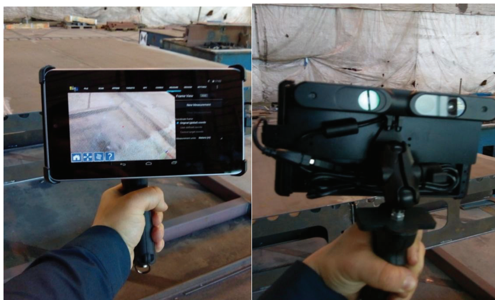
Figure 5.1. Handheld scanner from DotProduct (photo author, May 2018)
