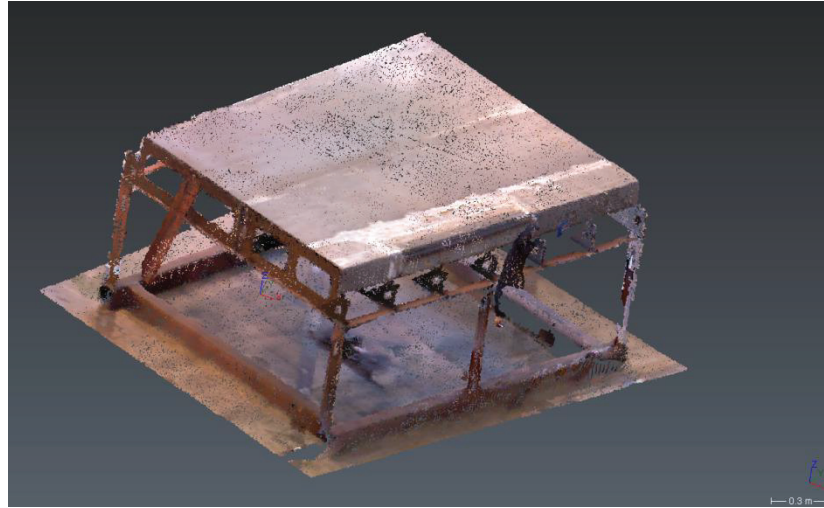
Figure 5.2. The result of the scanning with the DPI-7 from DotProduct
