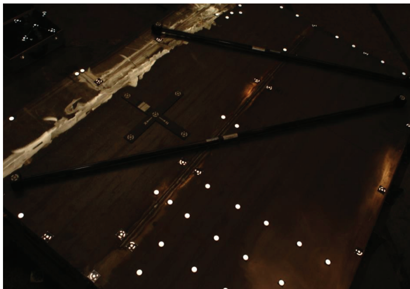
Figure 4.10. Location of the scale bars and the special coded marks fixed with the magnet to the steel detail for test measurements (photo author, May 2018)
