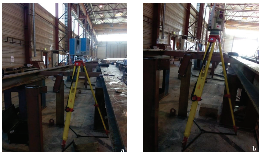
Figures 3.5 (a,b). Devices for laser scanning: Laserscanner Z+F Imager 5010 (a) and Leica Total Station TS-15 (b) (photos author, April 2018)
