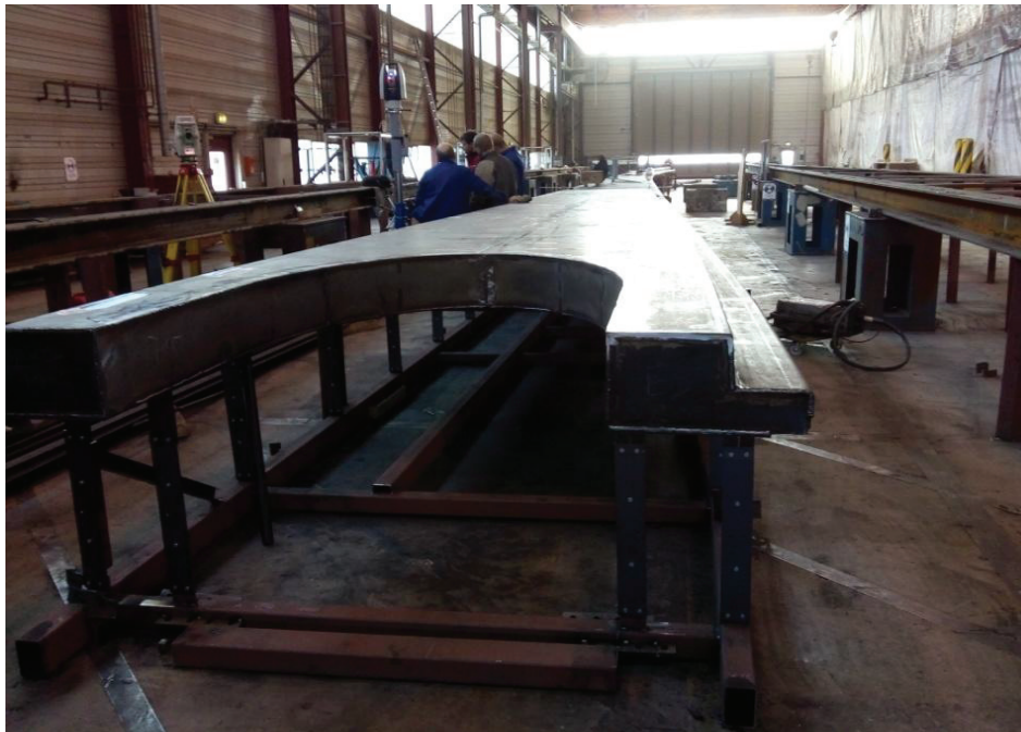
Figure 1.3. Connected cold and hot frame of the adhesive angle of the ship. The detail is located between two stands for hot frame. View from the section A (photo author, April 2018)
