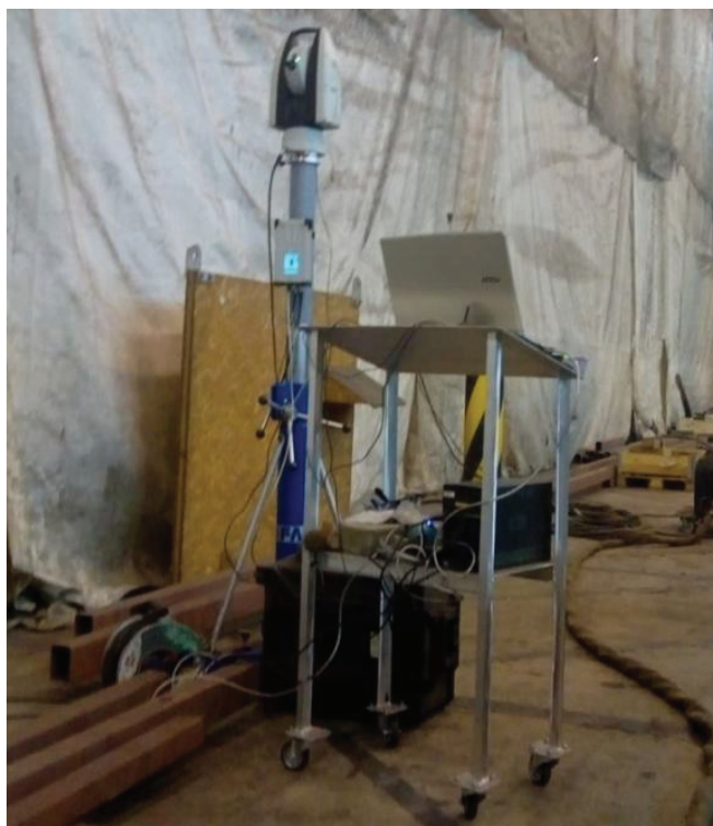
Figure 2.3. Leica Absolute Tracker AT960-LR in the work process (photo author, March 2018)
