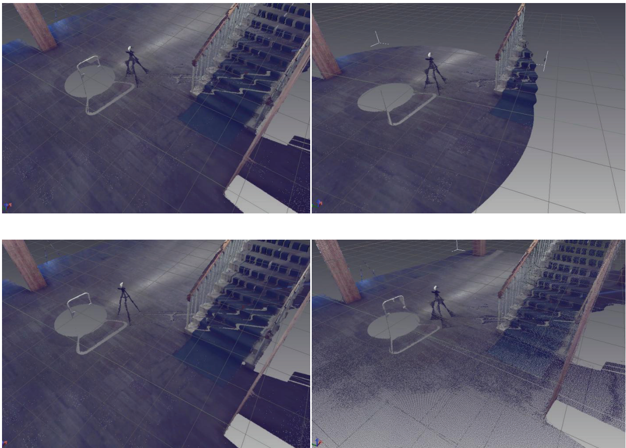
Abb. 46 ohne Filter (o.l.), Range from Scanner (o.r), Scanpoint Distance (u.l.), Uniform (u.r.)
