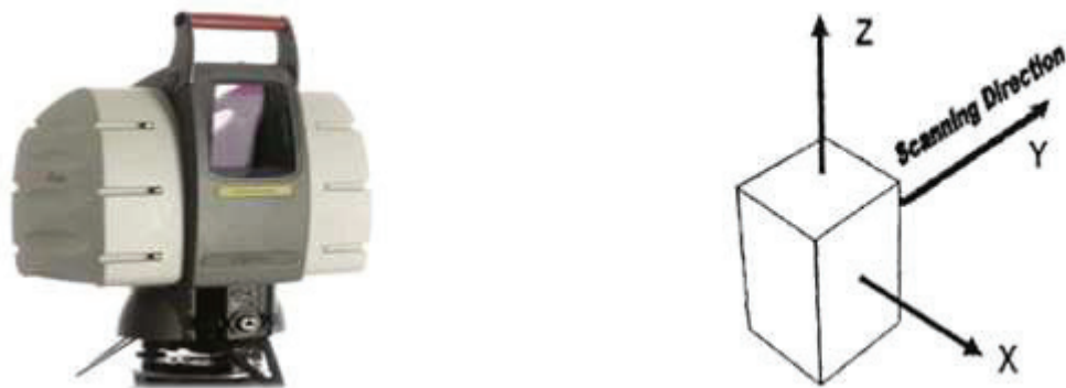
Figure 14 HDS 3000 and its default coordinate system [18]
