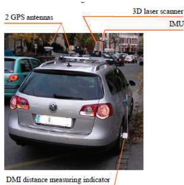
Figure 6 Components of Kinematic Laser Scanning
