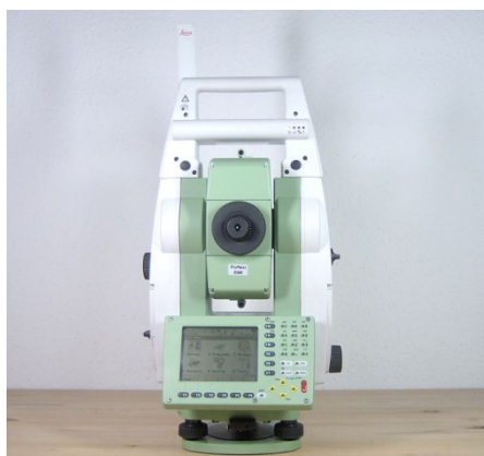
Abb. 27: Totalstation TCRP (Leica)
