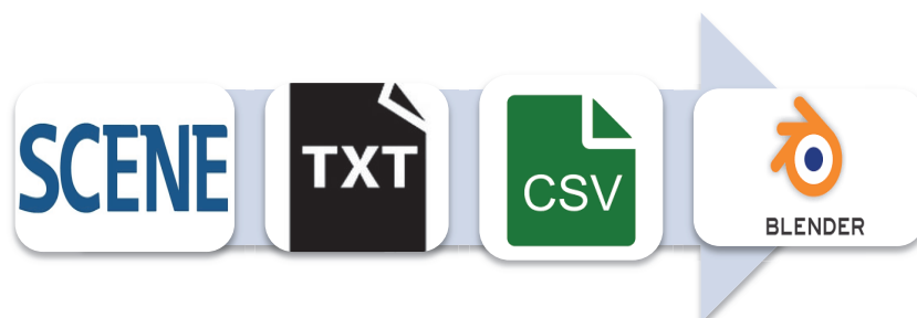
Figure 7.1: Scheme Of Importing XYZ Point Cloud In Blender Using CSV Mesh Importing
